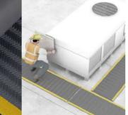
The Renolit Alkorplan Walkway is a waterproof membrane used for maintenance, access and emergency routes. It is laminated with flexible PVC and has a woven polyester reinforcement.
