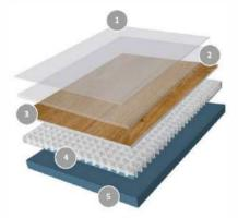
1. Hyperguard+ PUR Layer Easier cleaning and reduced scuff and dirt adherence 2. Wear Laver High performance for high-wear applications 3. Decor Layer Exclusive designs with incredible realism 4. Insulation Layer Provides acoustic absorption and ease of installation 5. High-Density Backing Adds stability and contributes to insulative properties
