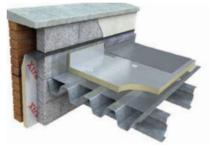
Xtratherm FR/ALU is a high performance flat roof insulation board with vapourtight aluminium foil facings suitable for use with single ply membranes.
