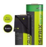
RESITRIX<sup>®</sup> SK Partial Bond is a partially self-adhesive, heat-weldable EPDM waterproofing membrane that allows permanent dissipation and equalisation of pressure. It is therefore particularly advantageous for substrates that are prone to movement or which contain residual moisture
