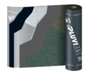
Pluvitec Specialtec is an APP modified bituminous waterproofing membrane with both composite polyester and fibreglass reinforcements providing both good mechanical characteristics and excellent dimensional stability.
