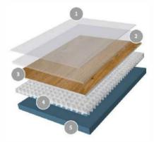
1. Hyperguard+ PUR Layer Easier cleaning and reduced scuff and dirt adherence 2. Wear Layer with Chips Provides slip resistance for high wear applications 3. Decor Layer Exclusive designs with incredible realism 4. Insulation Layer Provides comfort absorption and ease of installation 5. High-Density Backing
