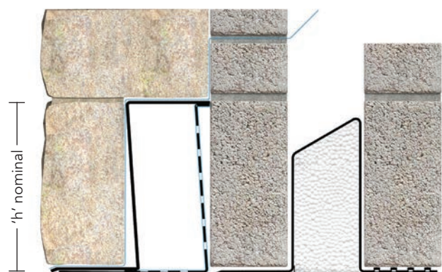
BOX/K-200 lintel shown with optional feature plate.
