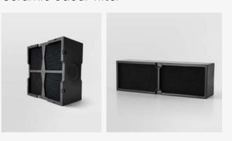
The ceramic filter is a modular charcoal filter that can be thermally regenerated in the oven every 2/3 months at 200° for 45 minutes, up to max 5 years. It allows for very high odour absorption efficiency and very high mechanical strength.
