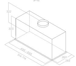
Lane is the invisible hood that blends perfectly into the kitchen's linearity. It features a modern design, high performance and offers excellent value for money. Moreover, it comes with a patented fastening system made up of 2 side clips, allowing the hood to be secured to the cabinet with only 2 screws from below, in less than one minute.
