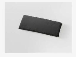
Odour filter with very high efficiency level >82%. Capable of regenerating itself and of lasting up to a maximum of 3 years in comparison to standard filters. To maintain such characteristics, the filter must be washed every 2 or 3 months with hot water and mild soap, or in the dishwasher at 65°C. and can be dried in the the oven for 10 minutes at 100°.
