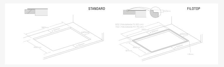
Recommended filotop dimensions: for different tolerances, respect the actual dimensions of the glass.
