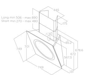
When activated, the central ring electronically shifts inward, thus allowing the hood to activate perimeter extraction.
