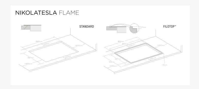
$^{st}$  Recommended filotop dimensions: for different tolerances, respect the actual dimensions of the glass.
