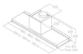
A very simple and essential design characterizes this appliance, which is completely hidden in the cabinet . It is equipped with a frontal visor that protects the door during cooking , conveying vapours through the extraction area.
