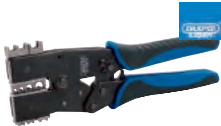
7 220mm Quick Change Ratchet Crimping Tool Expert Quality, made from carbon steel, Supplied with two sets of interchangeable hardened and tempered jaws. Chemically blacked finish with PVC grips. Suitable for crimping insulated terminals as follows: - red channel: 0.5 - 1.00mm, blue channel: 1.5 - 2.5mm and yellow channel: 4.0 - 6.0mm, and non - insulated crimps 1.5, 2.5, 6 and 10mm. Display packed.
