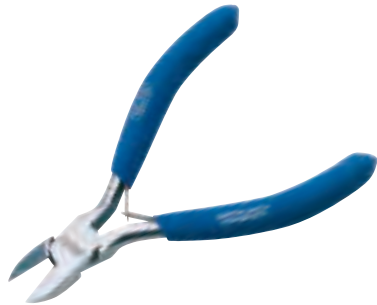
3 110mm Carbon Steel Diagonal Side Cutters Carbon steel, hardened and tempered with textured grips, captive double leaf springs and bevel cut induction hardened cutting edges. Display packed.
