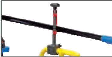
Safety device preventing users from operating the compressor when the safety cage is open
