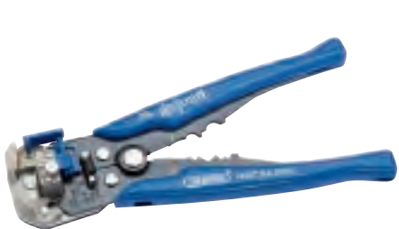
6 Dual Action Automatic Wire Stripper/Crimper, 210mm Professional or DIY use. Single motion stripping of wires/insulation and the crimping of insulated and non - insulated terminals. Wire stripping range 0.13 - 8.0mm/8 - 26AWG, crimping range 0.5 - 6mm/10 - 22AWG. Carbon steel blades, alloy steel jaws hardened and tempered, with plastic hand grips. Display packed.
