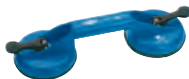
3 Twin Suction Cup Lifter For the easy lifting of smooth flat surface materials, i.e. glass, marble etc. Manufactured from tough plastic with rubber suction cups. Suction cups 118mm diameter. Maximum lift 40kg; safe working load (S.W.L.) 20kg. Display packed.
