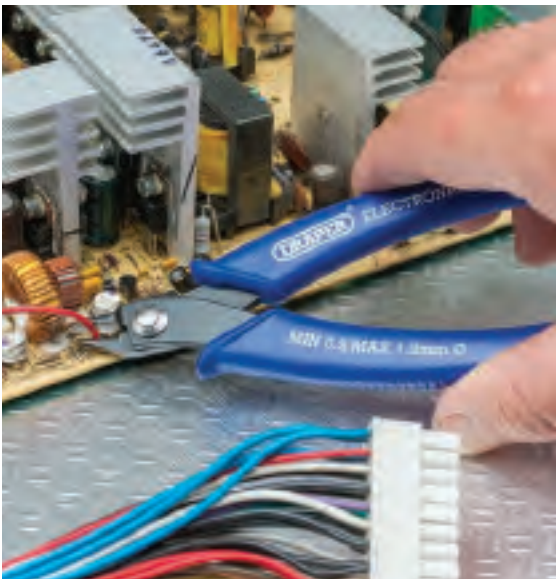
8 Thin Jaw Electronics Nippers, 130mm Carbon steel, hardened and tempered for cutting copper wire up to 1.2mm diameter. Chemically blacked finish with soft grips and limiter feature. Display packed.
