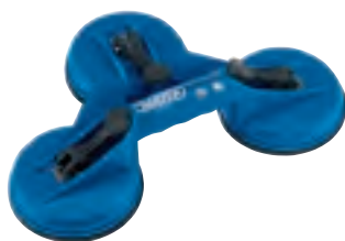
4 Triple Suction Lifter For the easy lifting of smooth flat surface materials, i.e. glass, marble etc. Manufactured from tough plastic with rubber suction cups. Suction cups 118mm diameter. Maximum lift 75kg; safe working load (S.W.L.) 37.5kg. Display carton.
