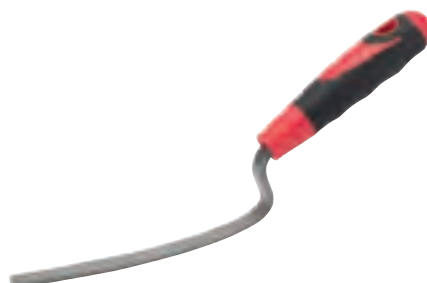
2 Draper Redline® Brick Jointer Trowel Designed to finish the mortar joints between bricks. Suitable for 13mm joints. Manufactured from hardened and tempered carbon steel.
