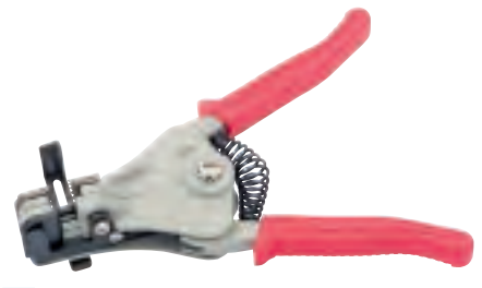
5 Automatic Wire Strippers Automatic clamping action and length gauge facility ensure stripped ends are uniform. The replaceable blades are accurately notched and honed to strip five insulation or wire diameters, 1.0, 1.6, 2.0, 2.6 and 3.2mm. Spring-loaded moulded grip handles. Display packed.
