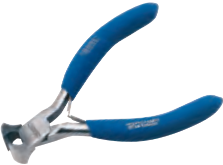
4 105mm Carbon Steel End Cutting Pliers Carbon steel, hardened and tempered with textured grips, captive double leaf springs and bevel cut induction hardened cutting edges. Display packed.
