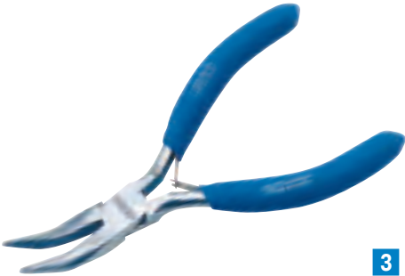
2 125mm Carbon Steel Bent Nose Pliers Carbon steel, hardened and tempered with textured grips and captive double leaf springs. Jaws angled up to 30°. Display packed.
