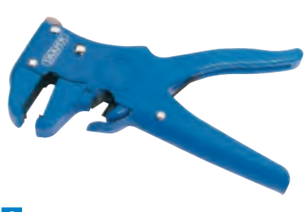
3 Automatic Wire Stripper/Cutter, 175mm Steel body with ABS moving handle. Wire stripper and cable cutter hardened and tempered SK5 steel. Strips and cuts single - layer wire from 0.2 - 4mm diameter. Also cuts 11mm wide and strips 14mm wide ribbon cable. Safety guard on wire cutter. Display packed.
