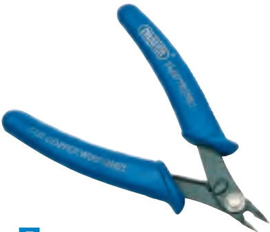
7 130mm Flush Cut Electronics Nippers Carbon steel, hardened and tempered for cutting copper wire up to 1.2mm diameter. Chemically blacked finish with soft grips and limiter feature. Display packed.
